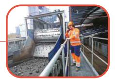
**4.** Once the metal has been weighed or broken, it is sorted into different materials in a number of different ways, including using water to separate heavy and light materials, or lasers and magnets to detect different metals. We have a seperate recycling centre for plastics.
